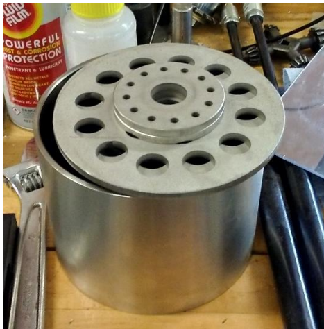
Figure 25. Print and impression roller parts prior to completion.
