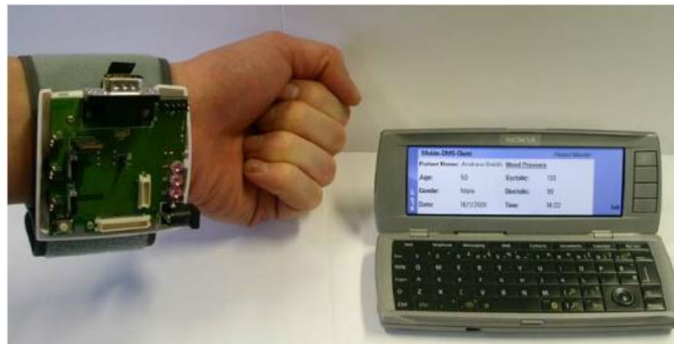
Figure 4. A patient monitoring device which transmits blood pressure readings, etc. [18]
