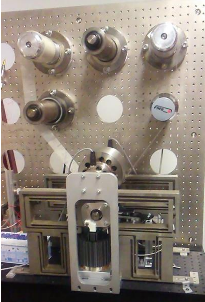
Figure 41. R2R setup in action: running web tension experiment. Note that lower right idler roller has been swapped for tension measuring roller.
