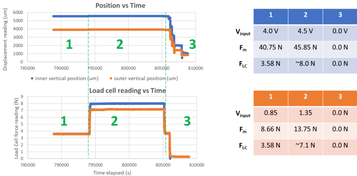
Figure 45. Plots from load cell calibration experiment. Tables display force data from both sides' VCAs.
